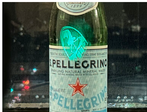
Demonstration of fully transparent display, creating bright green University of Southampton stag logo. (Photo provided by Smith Displays)
